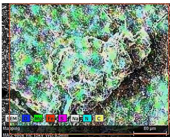
Figure 9 - EDS micrograph of MF41 with MO - 400X. Source: Author
